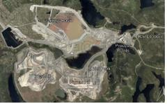
Phase 1 of the Bloom Lake Mine was commissioned in March 2010 and consists of an open pit truck and shovel mine, a concentrator that utilizes single-stage crushing, an autogenous mill and gravity separation to produce iron concentrate. From the site, concentrate is transported by rail to a ship loading port in Pointe-Noire.
